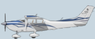
Cessna 182T Skylane - “Firespotter” Roles: Reconnaissance, supervision, utility. Single piston engine. Three passengers. Commonly used for fire spotting patrols. 270km/h, 230hp.
