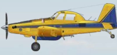
Air Tractor AT802F - “Bomber” Role: Fire bombing. Single engine, turbo prop air tanker. 3200 litre capacity. Drops water, foam, gel or fire retardant solutions. 350km/h, 1600hp
