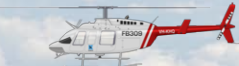
Bell 206L-3 LongRanger - “Firebird” Roles: Supervision, reconnaissance, utility. Single turbine engine. Six passengers. 220km/h, 650hp.
