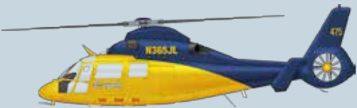
Eurocopter AS365N2 Dauphin - “Helitak” Roles: Fire crew insertion, firebombing, transport, utility. Twin turbine engine. Eight Passengers. 270KG, 100m winch. 1025 litre capacity bucket. 260km/h, 1500hp
