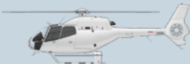
Eurocopter EC120B Colibri - “Firebird” Roles: Supervision, reconnaissance, utility. Single turbine engine. Four passengers. 220km/h, 500hp
