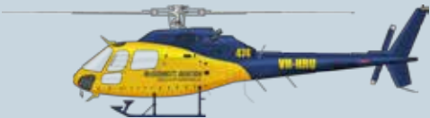
Eurocopter AS355F1 Twin Squirrel - “Firebird” Roles: Firebombing, supervision, utility. Twin turbine engines. Five passengers. 680 litre capacity bucket. 230km/h, 840hp.
