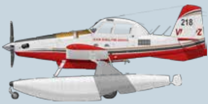
Air Tractor AT802F Fireboss - “Bomber” Roles: Firebombing. Amphibious, single engine turbo prop air tanker. 3200 litre capacity. Scoops water from lakes and rivers, adds foam, gel before dropping. 275km/h, 1600hp
