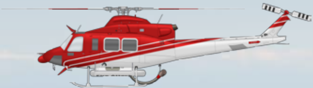
Bell 412SP - “Helitak” Roles: Firebombing, fire crew insertion, transport, utility. Twin turbine engine. 10 passengers. 270KG, 75m winch. 1400 litre capacity belly tank. 225km/h, 1800hp.
