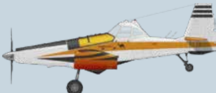
PZL M18T (Hubler) Dromader - “Bomber” Role: Fire bombing. Single engine, turbo prop air tanker. 2375 litre capacity. Drops water, foam, gel or fire retardant solutions. 230km/h, 1000hp
