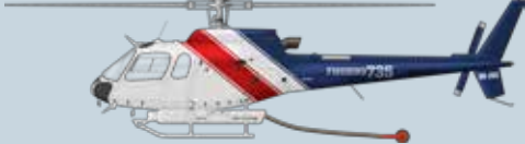
Eurocopter AS350B3 Squirrel - “Firebird” Roles: Firebombing, supervision, fire crew insertion, utility. Single turbine engine. Five passengers. 1100 litre capacity bucket or belly tank. 200km/h, 850hp.
