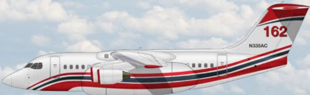
Avro RJ85 airtanker - “Bomber” Role: Firebombing. Four turbo fan engines. Two pilots. 11,350 litre retardant capacity tank. Drops foam, gel or fire retardant solutions. 680km/h, 12,700kg thrust.
