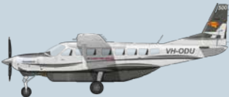
Cessna 208B Grand Caravan - “Birddog” Roles: Supervision, reconnaissance, transport, utility. Single turbine engine, high wing. Nine passengers. 300km/h 675hp
