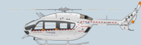
Eurocopter EC145 - “Helitak” Roles: Fire crew insertion, firebombing, transport, utility. Twin turbine engine. Eight Passengers. 270KG, 91m winch. 910 litre capacity bucket. 220km/h, 1500hp
