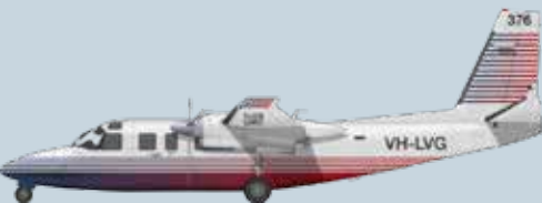
Rockwell Turbo Commander 690B - “Birddog” Roles: Supervision, reconnaissance, transport, utility. Twin turbine engine, high wing. Five passengers. 500km/h 1430hp
