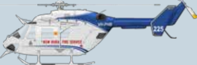
MBB/Kawasaki BK 117 - “Helitak” Roles: Fire crew insertion, firebombing, transport, utility. Twin turbine engine. Eight Passengers. 270KG, 75m winch. 900 litre capacity bucket. 215km/h, 1500hp
