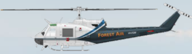
Bell 204B - “Helitak” Roles: Firebombing, transport, utility. Single turbine engine. 14 passengers. 1290 litre capacity long-line bucket. 185km/h, 1400hp
