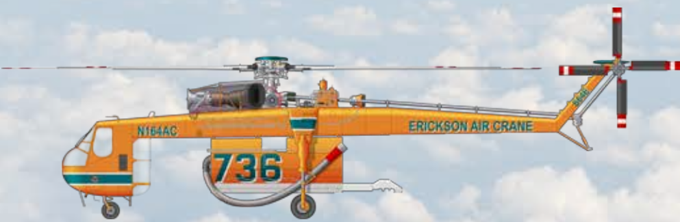
Erickson S64E Airplane - “Helitak” Role: Firebombing. Twin turbine engine. Two Pilots. No passengers. Hover Fill and sea skimming snorkels. 7560 litre capacity tank 215km/h, 9000hp.
