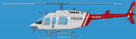
Bell 206L-3 LongRanger – “Firebird” Roles: Supervision, reconnaissance, utility. Single turbine engine. Six passengers. 220km/h, 650hp.
