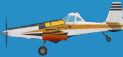
PZL M18T (Hubler) Dromader – “Bomber” Role: Fire bombing. Single engine, turbo prop air tanker. 2375 litre capacity. Drops water, foam, gel or fire retardant solutions. 230km/h, 1000hp
