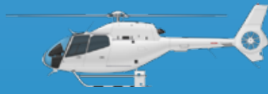
Eurocopter EC120B Colibri – “Firebird” Roles: Supervision, reconnaissance, utility. Single turbine engine. Four passengers. 220km/h, 500hp
