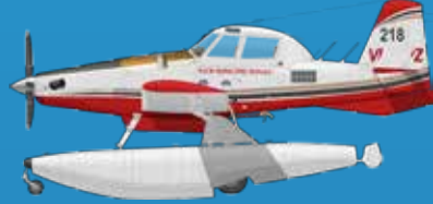
Air Tractor AT802F Fireboss – “Bomber” Roles: Firebombing, amphibious, single engine, turbo prop air tanker. 3200 litre capacity. Scoops water from lakes and rivers, adds foam, gel before dropping. 275km/h, 1600hp
