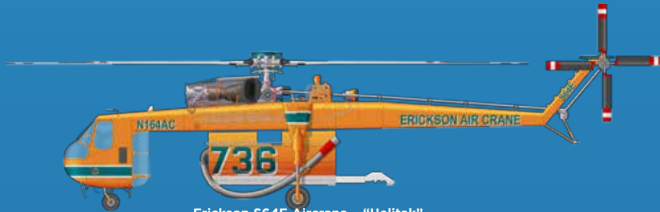
Erickson S64E AirCrane – “Helitak” Role: Firebombing. Twin turbine engine. Two Pilots. No passengers. Hover Fill and sea skimming snorkels. 7560 litre capacity tank 215km/h, 9000hp.
