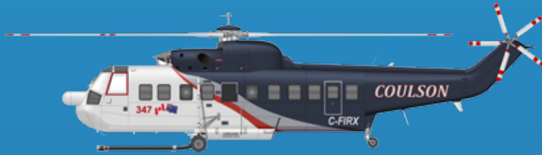
Sikorsky S61N – “Helitak” Roles: Firebombing, fire crew insertion, transport. Twin turbine engines. Two pilots. Eighteen passengers. 4000 litre capacity belly tank or 2850 litre power fill bucket. 225km/h, 3000hp.
