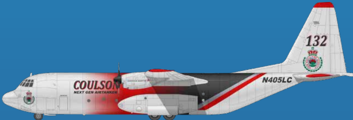
Lockheed Martin L100-30 airtanker – “Bomber” Role: Firebombing. Four turbo props engines. Two pilots and one flight engineer. 15450 litre retardant capacity tank. Drops foam, gel or fire retardant solutions. 545km/h (loaded), 18,000hp.
