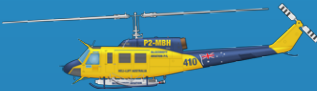
Bell 214B Big Lifter – “Helitak” Roles: Firebombing, transport. Single turbine engine. Fourteen passengers. 2650 litre capacity belly tank or bucket. 240km/h, 2950hp
