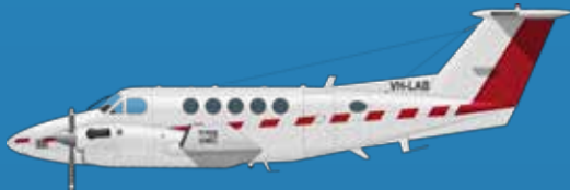
Beechcraft King Air - B200T Roles: Fire Scanning, reconnaissance, utility. Twin engine turboprop. Single pilot, one system operator. Infrared and multispectral line scanner, satellite broad band data transmission, 2+ fire agency radios, Satellite tracking. 450km/h.
