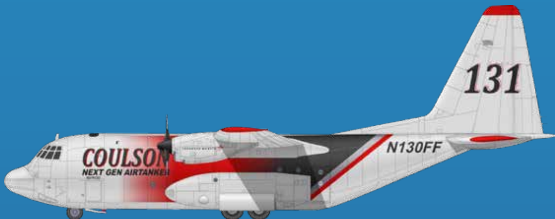
Coulson C130Q airtanker – “Bomber” Role: Firebombing. Four turbo props engines. Two pilots and one flight engineer. 15450 litre retardant capacity tank. Drops foam, gel or fire retardant solutions. 545km/h (loaded), 18,000hp.
