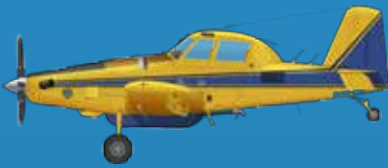
Air Tractor AT802F – “Bomber” Role: Fire bombing. Single engine, turbo prop air tanker. 3200 litre capacity. Drops water, foam, gel or fire retardant solutions. 350km/h, 1600hp
