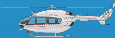
Eurocopter EC145 – “Helitak” Roles: Fire crew insertion, firebombing, transport, utility. Twin turbine engine. Eight Passengers. 270KG, 91m winch. 910 litre capacity bucket. 220km/h, 1500hp
