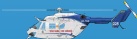
MBB/Kawasaki BK 117 – “Helitak” Roles: Fire crew insertion, firebombing, transport, utility. Twin turbine engine. Eight Passengers. 270KG, 75m winch. 900 litre capacity bucket. 215km/h, 1500hp
