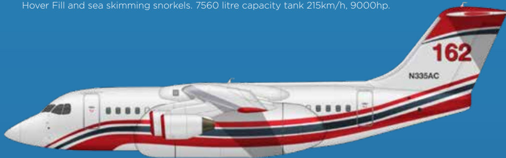
Avro RJ85 airtanker – “Bomber” Role: Firebombing. Four turbo fan engines. Two pilots. 11,350 litre retardant capacity tank. Drops foam, gel or fire retardant solutions. 680km/h, 12,700kg thrust.
