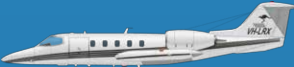
Gates Learjet 35A Roles: Fire Scanning, reconnaissance, utility. Twin engine turbofan. Two pilots, one system operator. Infrared and multispectral line scanner, satellite broad band data transmission, 2+ fire agency radios, Satellite tracking. 650km/h.
