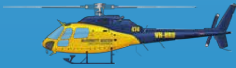
Eurocopter AS355F1 Twin Squirrel – “Firebird” Roles: Firebombing, supervision, utility. Twin turbine engines. Five passengers. 680 litre capacity bucket. 230km/h, 840hp.
