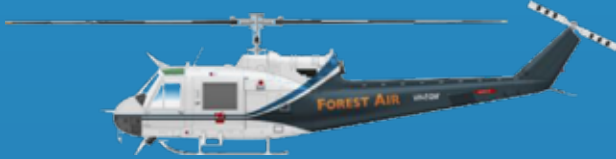
Bell 204B – “Helitak” Roles: Firebombing, transport, utility. Single turbine engine. 14 passengers. 1290 litre capacity long-line bucket. 185km/h, 1400hp
