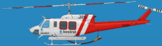
Bell 212 – “Helitak” Roles: Firebombing, fire crew insertion, transport, utility. Twin turbine engine. Fourteen passengers. Rappel equipment, 1475 litre capacity belly tank. 185km/h, 1800hp.
